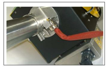
At the supplementary for gas sampling is possible to connect analyser of any manufacturer. By connecting a Mega System analyser with an Oxygen sensor (PARAMAGNETIC) and a Carbon Dioxide sensor (NDIR) is possible to calculate the density of the gaseous affluent in compliance with the actual regulation during the isokinetic sampling.
